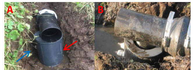
Figure 2: A: Flowcap with SorbiCells (blue arrow) and outlet (red arrow). B: Flowcap partially under water.
